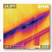
The thermal image shows a badly sealed ceiling causing cold air to leak into the building.
